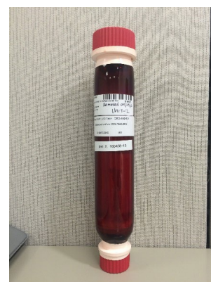
AMESA trap (contains XAD resin and spike)
