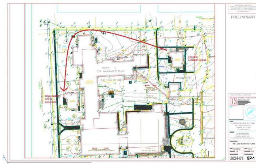
8.2.2.A –Site Plan – Building Re-location (note: not illustrative of building moving route.)
